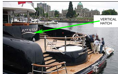
Fig. 12 Attessa III – after refit with new hatches in Victoria, BC, Canada
